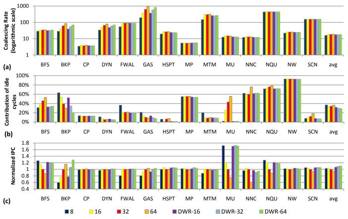
Figure 4. Comparing (a) Coalescing rate, (b) Idle cycle share and (c) Performance for different configurations of DWR and processors using different warp sizes. Each configuration of DWR is notated by DWR-x where x denotes the largest warp size.
