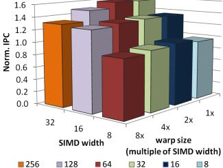
Figure 1. Warp size impact on performance for different SIMD widths, normalized to 8-wide SIMD and 2x warp size.
