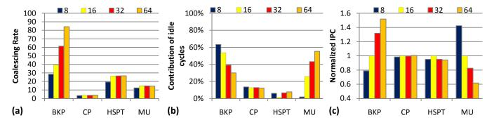
Figure 2. (a) Coalescing rate, (b) Idle cycle share and (c) Performance under different warp sizes. IPC is normalized to a GPU using 16 threads per warp.
