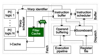
Fig. 3. Modifications made to the instruction fetch stage to implement an FC-enhanced SM.
