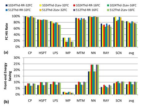
**Fig. 5.** Sensitivity for a) FC hit rate and b) front-end energy reduction to the multithreading depth (1024 and 512), warp scheduling policy (RR for round-robin and 2Lev for two-level scheduler), and FC size (32 and 16) for different benchmarks.
