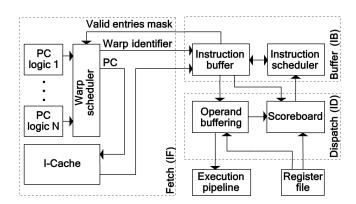
Fig. 1. The microarchitecture of SM's front-end.
